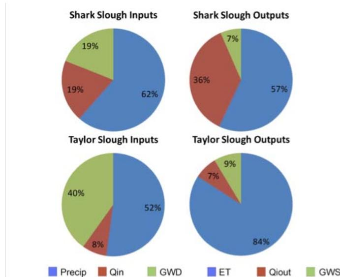
**Figure 5.6:** Pie charts of water budget components in Shark and Taylor Sloughs. Inputs include precipitation (blue), surface water inflow (red), and groundwater discharge (green). Outputs consist of evapotranspiration (blue), surface water outflow (red), and groundwater seepage (green). Values represent the average percentages of each component for Taylor Slough on a monthly basis between Jan. 2008 – July 2009, and on an annual basis in Shark Slough between 2002-2008.
