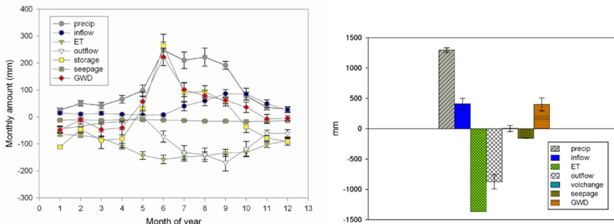
**Figure 8.19:** Left panel shows monthly water budget components while right panel shows annual water budget components. Results shown here are averages over 2002-2008. The combination Penman-Montieth model of evapotranspiration (Shuttleworth 1992) has been chosen amongst other models for the water budget shown here. This model has further been modified to account for seasonal water limitation (drying up, increasing salinity) that can decrease evapotranspiration in the dry season.
