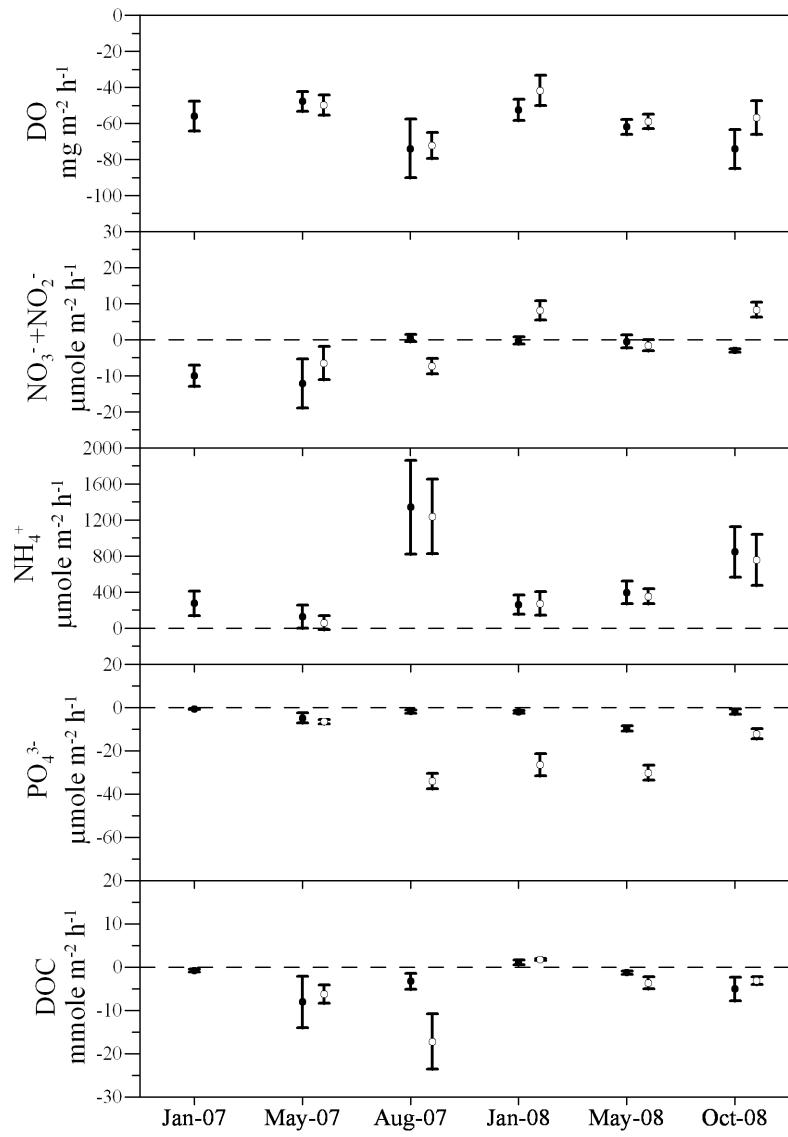
**Figure 3.2b.** Plot of mean fluxes ( $\pm \text{SD}$ ) of DO,  $\text{NO}_3^- + \text{NO}_2^-$ ,  $\text{NH}_4^+$ , SRP, and DOC from sediment cores collected at Pond 1. ● as Control, and ○ as P addition. N = 10 in Jan. 2007 and 5 thereafter.
