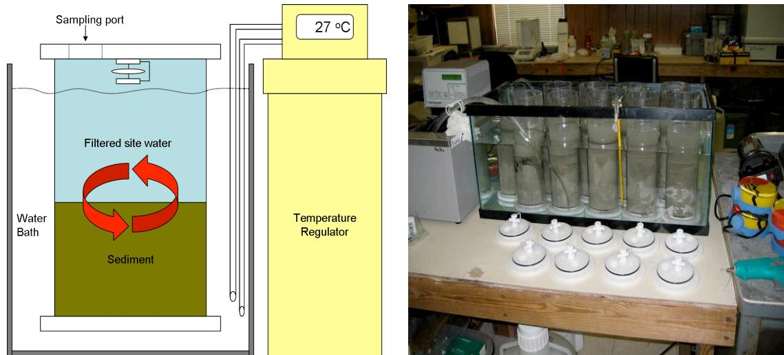
**Figure 3.1.** Illustration of core incubation scheme used to measure nutrient exchange along the Taylor River mangrove ecotone. The photo on the right is of a set of sediment cores collected from a mangrove pond near TS/Ph-7 (Pond 1).
