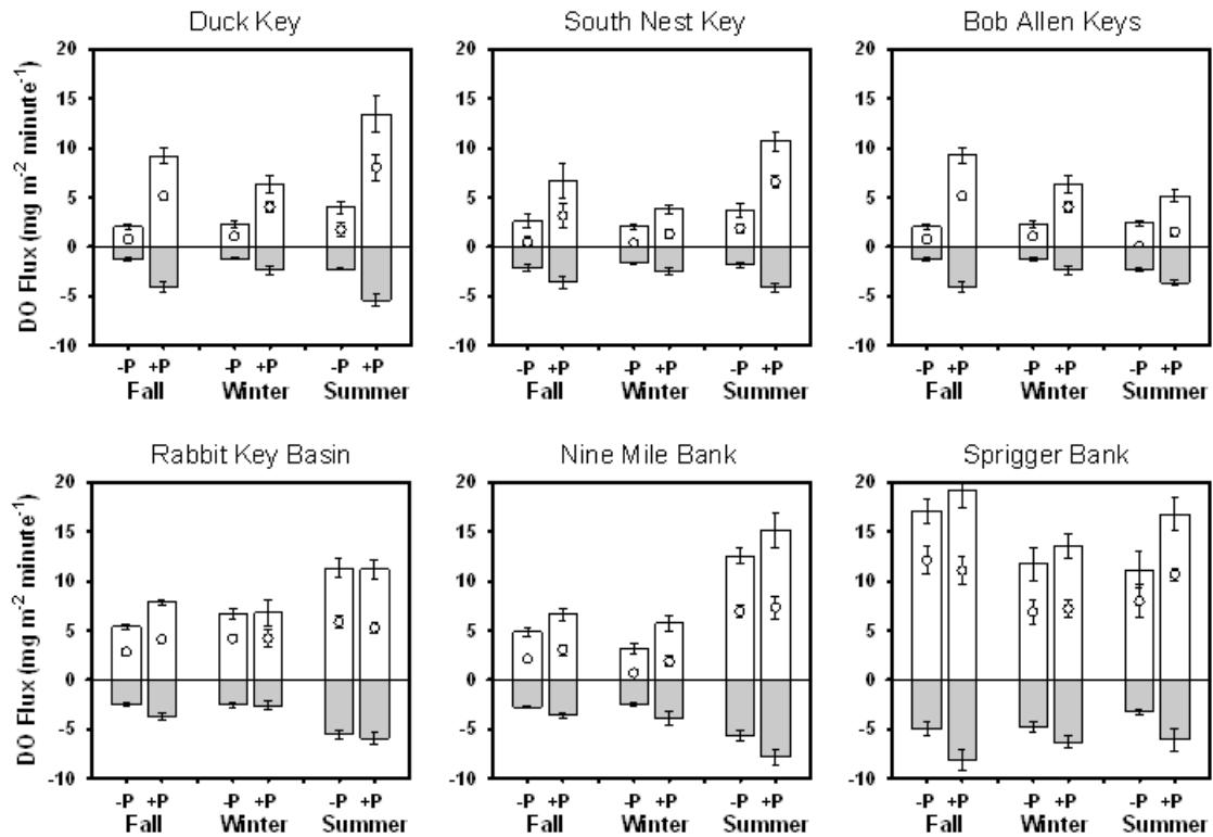
**Figure 1.7.** Dissolved Oxygen fluxes measured in closed chambers in situ. Bars above the zero-reference represent gross O<sub>2</sub> production in full daylight. Bars below the zero reference represent O<sub>2</sub> consumption in the dark. Bullets represent net O<sub>2</sub> production. Whiskers represent 1 SE.
