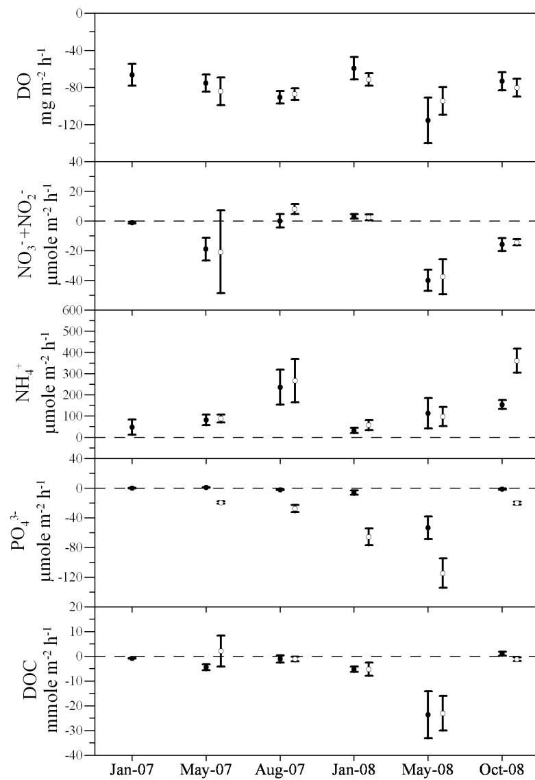
**Figure 3.2c.** Plot of mean fluxes ( $\pm$ SD) of DO,  $\text{NO}_3^- + \text{NO}_2^-$ ,  $\text{NH}_4^+$ , SRP, and DOC from sediment cores collected at Eastern Little Madeira Bay. ● as Control, and ○ as P addition. N = 10 in Jan. 2007 and 5 thereafter.
