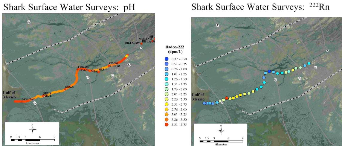
**Figure 5.1.** Surface water pH (left) and  $^{222}\text{Rn}$  (right) activity measured in Shark Slough between May 29, 2009 and April 5, 2009. Higher  $^{222}\text{Rn}$  levels tended to co-occur with lower pH values, possibly indicating groundwater discharge.
