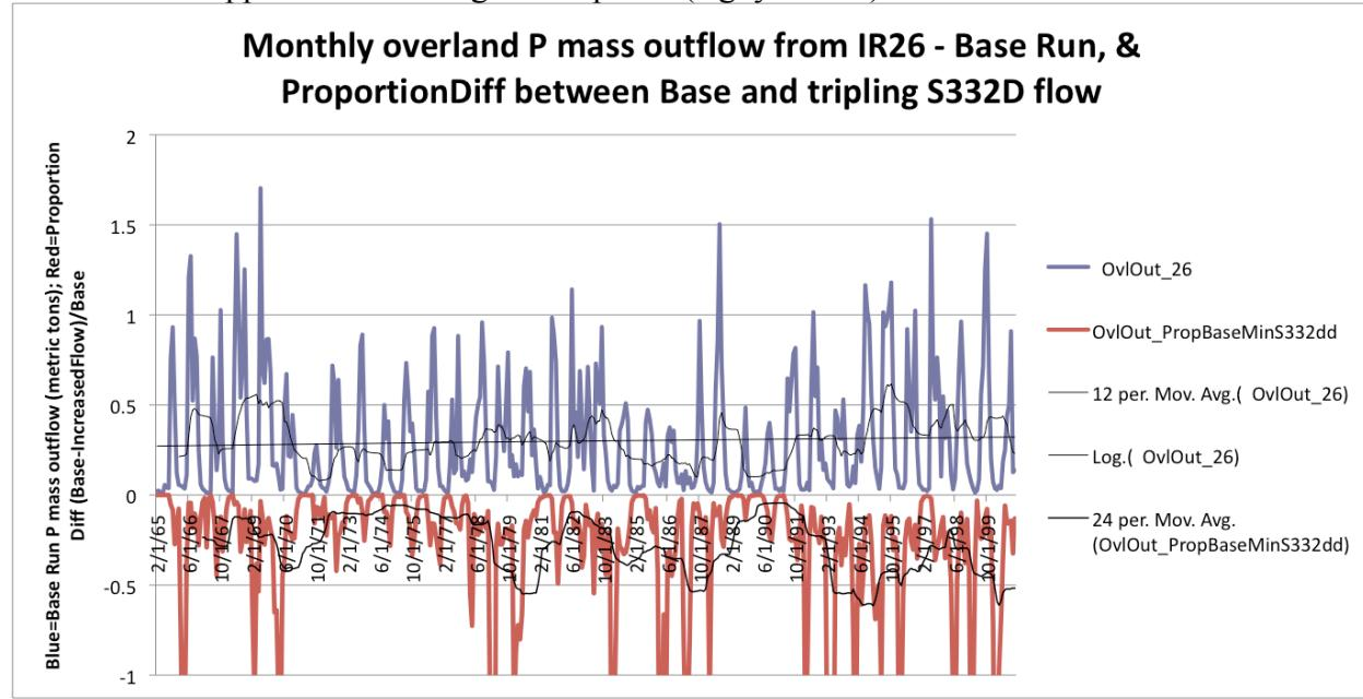
**Figure 8.4.** Proportional differences between ELM simulated P outflow for a future baseline case versus that of a future scenario with increased (tripled) inflows into the southern Everglades (through one structure (S-332D) upstream of the Taylor River region).
