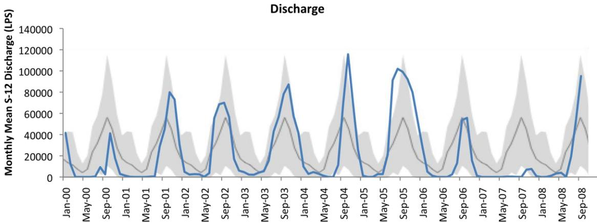
**Figure IIA.2.** Mean monthly discharge rates for water entering Shark River Slough (ENP) through the four S-12 structures along Tamiami Trail for 2000-2008 (blue line), 30-year mean discharge rates (gray line) and the 10<sup>th</sup> and 90<sup>th</sup> percentile values about that mean (gray shading).
