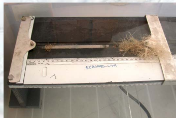
Figure 4. "LAMA" with Mylar leaf fouled by Polysiphonia binneyi , Duck, 73 days
