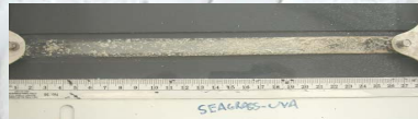
Figure 3. Light attenuation measurement apparatus, "LAMA", with Mylar leaf fouled by diatoms and adhered sediment, Bob Allen, 71 days
