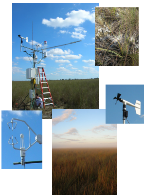
Figure 3. Images of the short hydroperiod Taylor Slough site (located at LTER site TS/Ph 1b) with the eddy covariance and meteorological systems.
