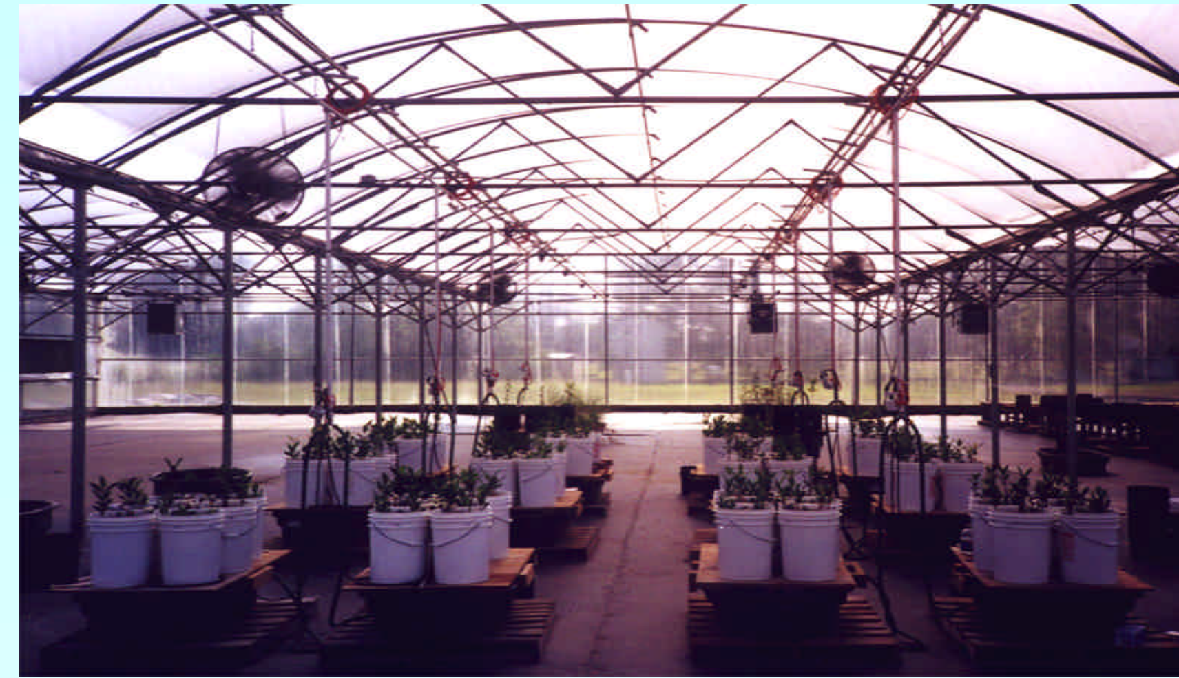
Fig 1. Experimental layout showing the tidal tables in which each white bucket represents an experimental unit. They host saplings of either Rhizophora or Laguncularia .
