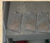
Figure 5: Represents the 6.35mm white nylon mesh bags used for the macroinvertebrate treatment (large mesh).
