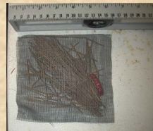
Figure 4: Represents the 1mm mesh fiberglass screening bags used for both the open air and soil surface treatment (small mesh).
